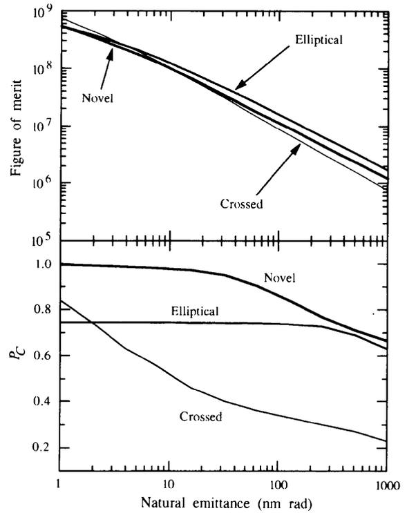
Figure 8 Emittance dependence of figure of merit and  $P_C$  for the elliptical, crossed and novel undulators.
