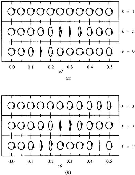
**Figure 4** Angular distribution of polarization obtained from the novel undulator for the (a)  $(4n + 1)$ th and (b)  $(4n + 3)$ th harmonics. The arrows in each ellipse show the direction of rotation.
