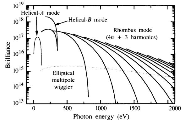
Figure 9 Peak brilliance obtained from the proposed device for three modes of operation and an example of a spectrum obtained from an elliptical multipole wiggler. The natural emittance is assumed to be 5 nm rad in each case.
