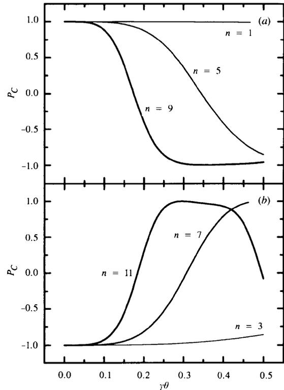
**Figure 5** Angular distribution of the degree of circular polarization,  $P_C$ , for the (a)  $(4n + 1)$ th and (b)  $(4n + 3)$ th harmonics.
