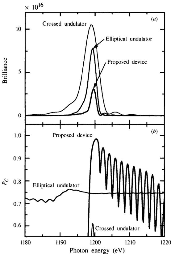
Figure 7 (a) Spectra and (b) degree of circular polarization,  $P_C$ , in the energy range between 1180 and 1220 eV.
