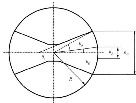
**Figure 2** Design parameters of the X-ray shutter drum; see equations (1)–(5).
