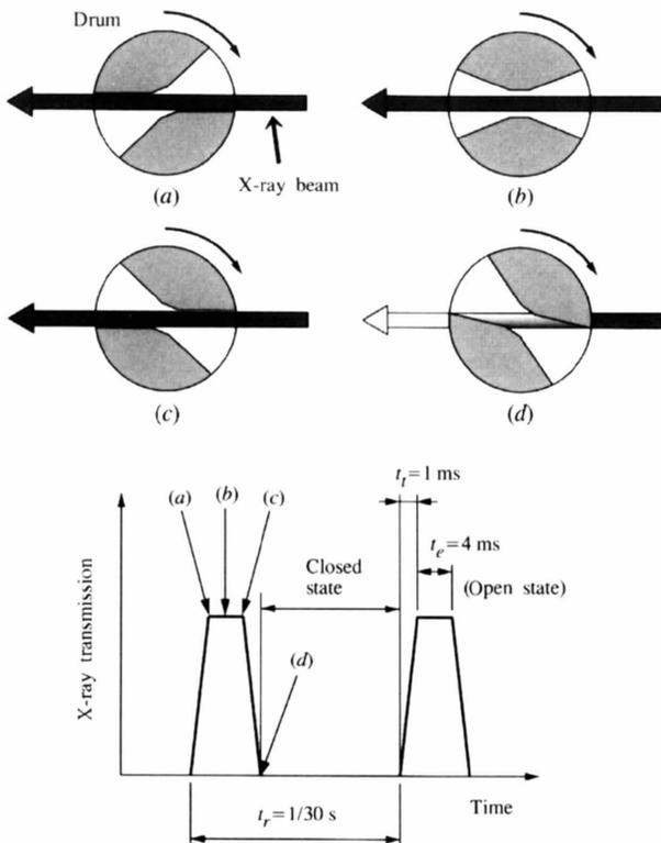
**Figure 1** Time-sequence drum rotation. (a) Beginning of the irradiation period; (b) centre; (c) end; (d) end of the transition and beginning of complete closing.  $t_r$  is the repetitive period of drum half rotation,  $t_e$  is the irradiation period of the X-rays, and  $t_t$  is the transition period between X-ray passing and stopping.
