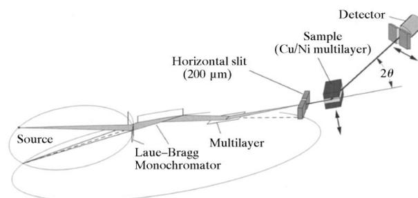
**Figure 1** Top view of the Laue–Bragg monochromator and multilayer combination. The experimental set-up on BM5 is sketched. The horizontal focusing of the bending-magnet radiation is achieved by meridionally bent Laue and Bragg crystals. The vertical focusing is provided by a bent multilayer. Residual strain profiles were measured by translating the sample through the line-focused beam monitoring the scattering angle. The parameters of the set-up are compiled in Table 1.
