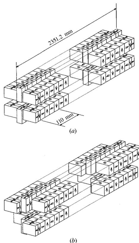
**Figure 1** Schematic figure of the UVSOR helical undulator in the (a) planar and (b) helical configurations.
