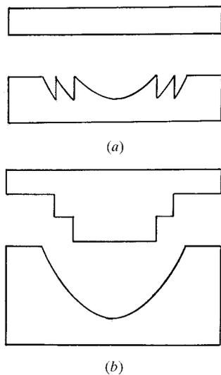
**Figure 7** Schematic diagram of two possible methods of reducing the increase of the vertical dimension of the diffracted beam shown in Fig. 6.
