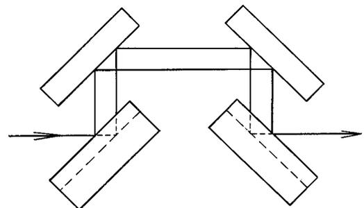
**Figure 8** A four-crystal dispersive  $(-, +, +, -)$  arrangement. The increase of the vertical dimension of the beam diffracted from the groove fabricated in the first or the second crystal is completely compensated by the groove fabricated in the third or the fourth crystal.
