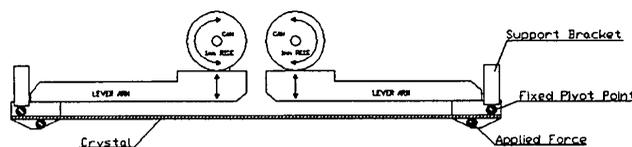
**Figure 1** Plan view of crystal bender showing the lever arms and cams that are used to apply a bending couple to the crystal.
