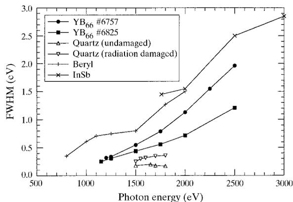
**Figure 7** FWHM of double-crystal rocking curves as a function of photon energy for two  $\text{YB}_{66}$  crystals #6767 and #6824 (Sc doped), and comparison with those for quartz (undamaged and damaged), beryl and InSb.
