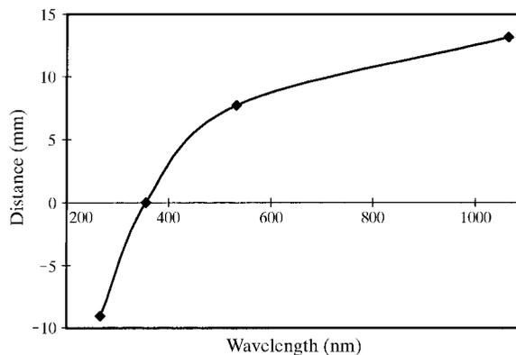
**Figure 8** Distance between the exit surface of the optical fiber and the focal position of the returning fluorescent light behind the surface, as a function of the wavelength of the emitted light.
