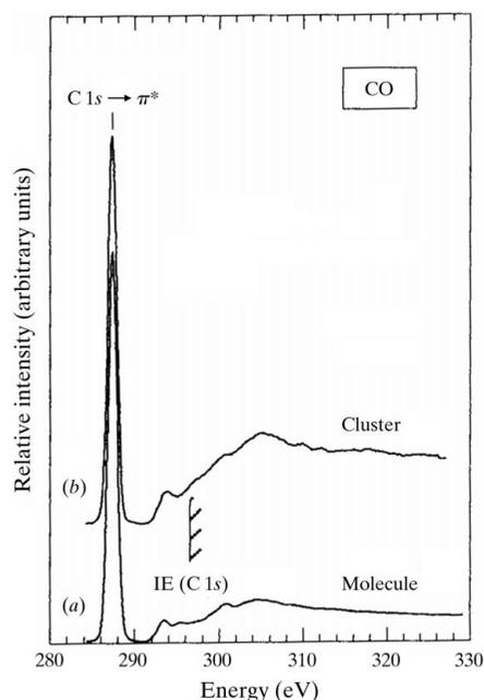
**Figure 1** (a) Total cation yield of neat CO recorded in the C 1s excitation regime. (b) Photoion yield of  $(\text{CO})_2^+$  recorded at  $\langle N \rangle \simeq 150$ . The vertical dashed line corresponds to the C 1s ionization energy [IE(C 1s) = 296.19 eV (Jolly *et al.*, 1984)].
