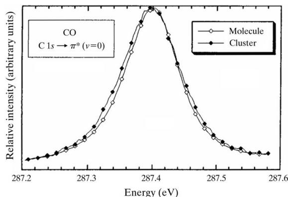
**Figure 2** Photoion yields of  $\text{C}^+$  (molecule) and  $(\text{CO})_2^+$  (cluster) recorded at  $\langle N \rangle \simeq 150$  in the C 1s  $\rightarrow \pi^*$  ( $\nu = 0$ ) regime. The lines connect the experimental data points. For clarity, every fifth data point is indicated by a diamond (molecule: open diamonds; clusters: filled diamonds).
