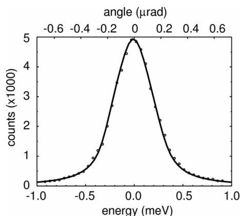
**Figure 4** Energy-resolution function for two silicon (12 12 12) crystals with a very modest asymmetry of  $43^\circ$  (asymmetry factor  $b \simeq 1.2$ ) oriented in a (+,+) geometry. The solid line is a fit using the theory of dynamical diffraction and is used to determine the silicon (12 12 12) structure factor.
