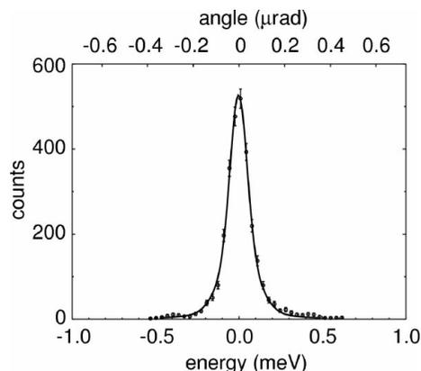
**Figure 5** Energy-resolution function for the ultra-high-resolution monochromator. The solid line is a simulation using the theory of dynamical diffraction with the structure factor determined from the result of Fig. 4 and its energy scale stretched by 27%. The FWHM is  $140 \mu\text{eV}$ .
