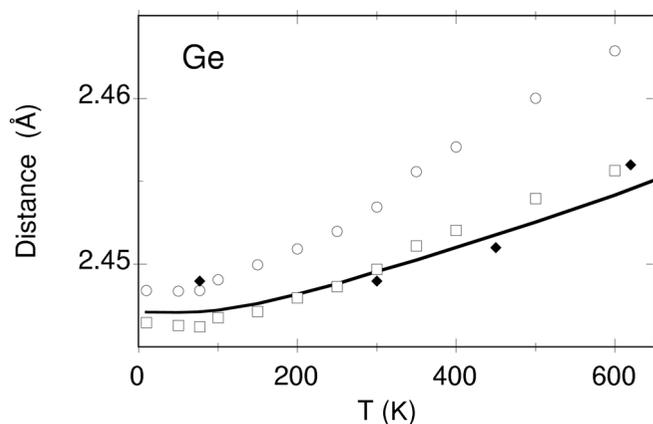
**Figure 9** Temperature dependence of the EXAFS cumulants for the first shell of germanium (Dalba *et al.*, 1999):  $C_1$  (squares) and  $C_1^*$  (circles). The continuous line is the crystallographic thermal expansion (Touloukian *et al.*, 1977). The diamonds are EXAFS distances quoted by Filipponi & Di Cicco (1995).
