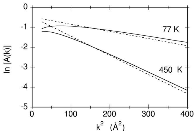
**Figure 5** Logarithm of  $A(k) = \exp(-2r/\lambda) \exp(-2k^2C_2)$  for the first shell of germanium. The experimental values of  $C_2$  at 77 and 450 K have been utilized. Dashed lines refer to a constant  $\lambda$  value of 10 Å, continuous lines to a more realistic  $k$ -dependence,  $\lambda = 2k/3 + 5/3$ .
