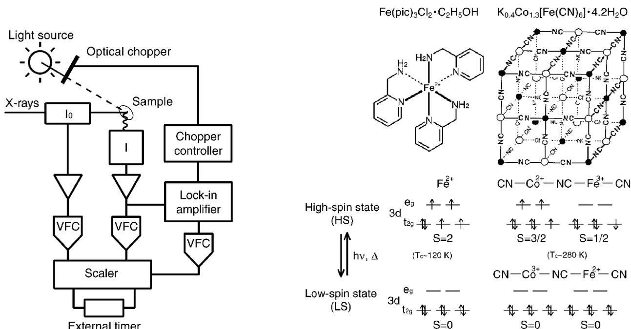
**Figure 3** Structures and orbital models of  $\text{Fe}(\text{pic})_3\text{Cl}_2 \cdot \text{C}_2\text{H}_5\text{OH}$ , **1**, and  $\text{K}_{0.4}\text{Co}_{1.3}[\text{Fe}(\text{CN})_6] \cdot 4.2\text{H}_2\text{O}$ , **2**.
