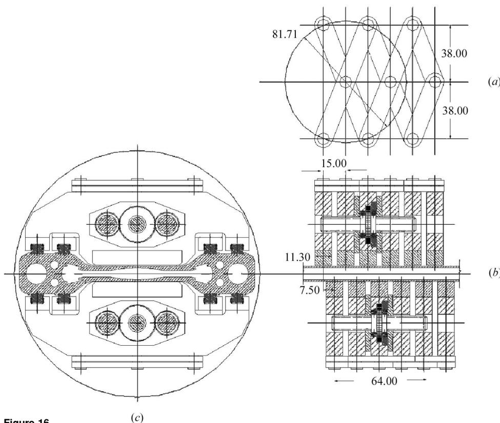
**Figure 16** Schematics of the various design components included in providing high-precision linear motion in the variable-period undulator. (a) Pantograph motion, (b) counter-screw motion and (c) supporting and guiding structure around the undulator-vacuum chamber. Dimensions are given in millimetres.
