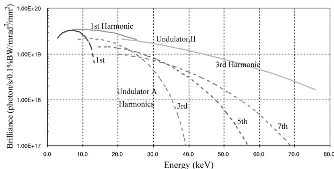
**Figure 10** The values of the brilliance of radiation as a function of the energy of the first and third harmonics delivered by undulator II (defined in Table 1) operating on a 7 GeV storage ring (see Table 2). The performance of undulator II is compared with that of the APS Undulator A, a 3.3 cm-period hybrid permanent-magnet undulator at the APS.
