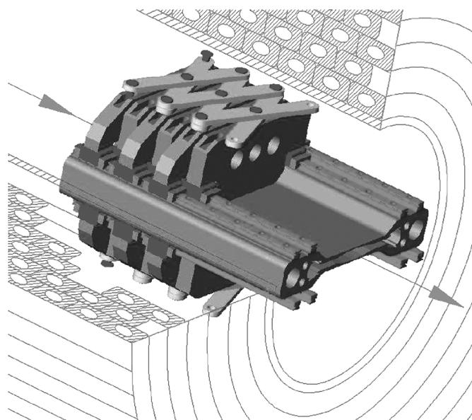
**Figure 17** A three-dimensional schematic of the driving mechanism for a variable-period undulator placed outside a straight-section vacuum chamber. A section of the magnetic solenoid is also shown.
