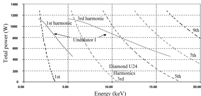
**Figure 7** The values of total power at various energies of the first and third harmonics delivered by undulator I (defined in Table 1) operating on a 3 GeV storage ring (see Table 2). The performance of undulator I is compared with that of U24, a 2.4 cm-period hybrid permanent-magnet undulator.
