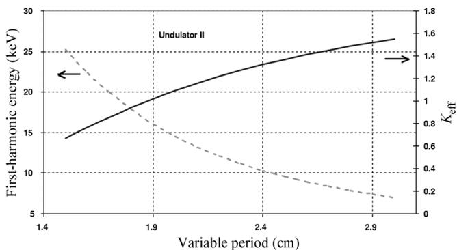
**Figure 9** The variation in the value of  $K_{\text{eff}}$  and the energy of the first harmonic as a function of the changing period of undulator II (defined in Table 1) operating on a 7 GeV storage ring (see Table 2).
