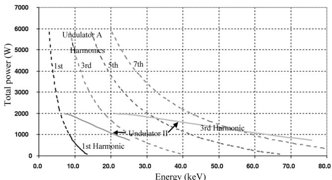
**Figure 11** The values of the total power at various energies of the first and third harmonics delivered by undulator II (defined in Table 1) operating on a 7 GeV storage ring (see Table 2). The performance of undulator II is compared with that of Undulator A, a 3.3 cm-period hybrid permanent-magnet undulator at the APS.
