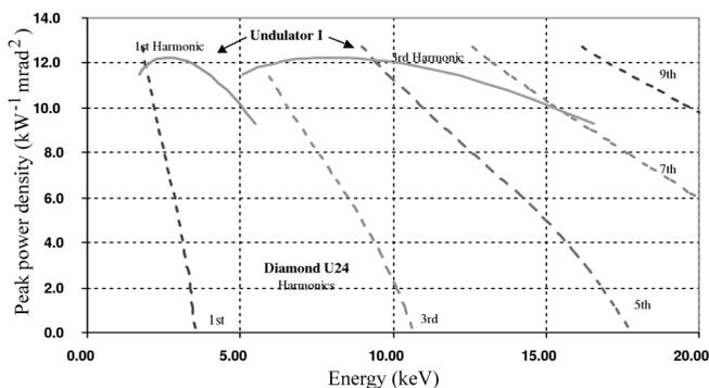
**Figure 8** The values of peak power density at various energies of the first and third harmonics delivered by undulator I (defined in Table 1) operating on a 3 GeV storage ring (see Table 2). The performance of undulator I is compared with that of U24, a 2.4 cm-period hybrid permanent-magnet undulator.
