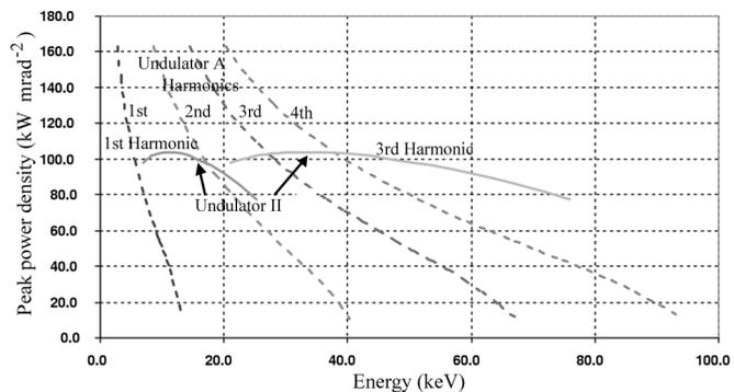
**Figure 12** The values of peak power density at various energies of the first and third harmonics delivered by undulator II (defined in Table 1) operating on a 7 GeV storage ring (see Table 2). The performance of undulator II is compared with that of Undulator A, a 3.3 cm-period hybrid permanent-magnet undulator at the APS.
