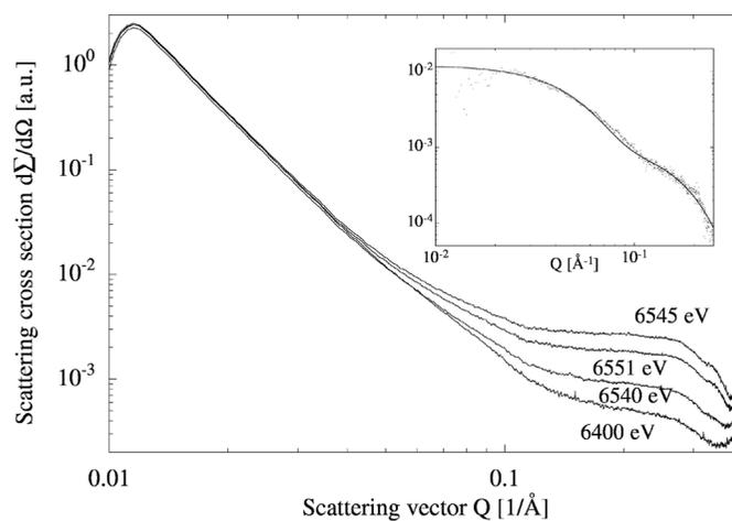
**Figure 7** Scattering curves of the entire *in situ* cell, obtained at four different X-ray energies.
