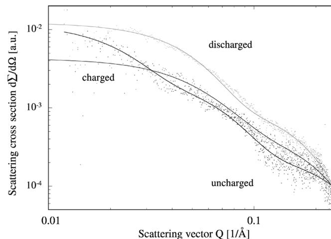
**Figure 8** Scattering curves of manganese oxide in electrode matrix for three different states of charge.
