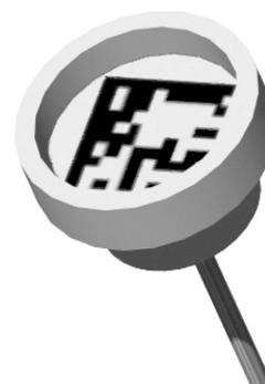
**Figure 6** Two-dimensional data matrix code for sample identification applied to the bottom of the Hampton-type magnetic caps.
