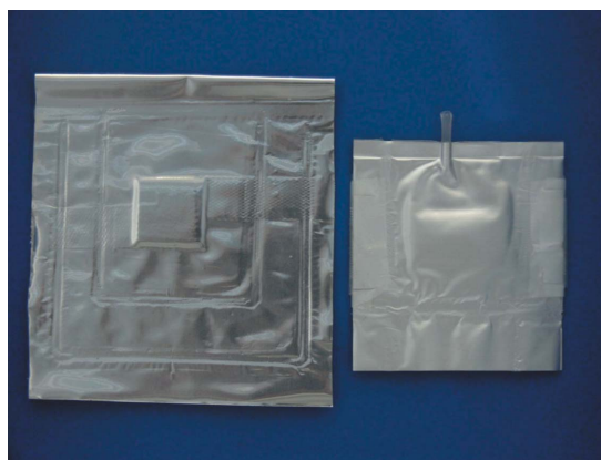
Figure 2 The two types of ‘coffee bag’ cells. On the left is the standard cell sealed in the machine; on the right the cell with a straw, sealed by hand.
