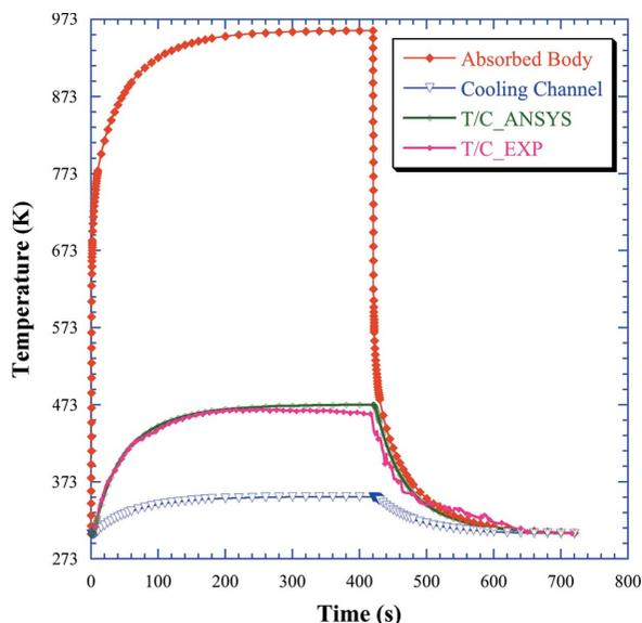
**Figure 8** Transient nodal solutions of the maximum temperatures on the absorbing body and the cooling surface when the absorbed power is 650 W. The measurements of the reference temperature (T/C\_EXP) and the nodal solutions (T/C\_ANSYS) at the location of the K-type thermocouple are also shown.
