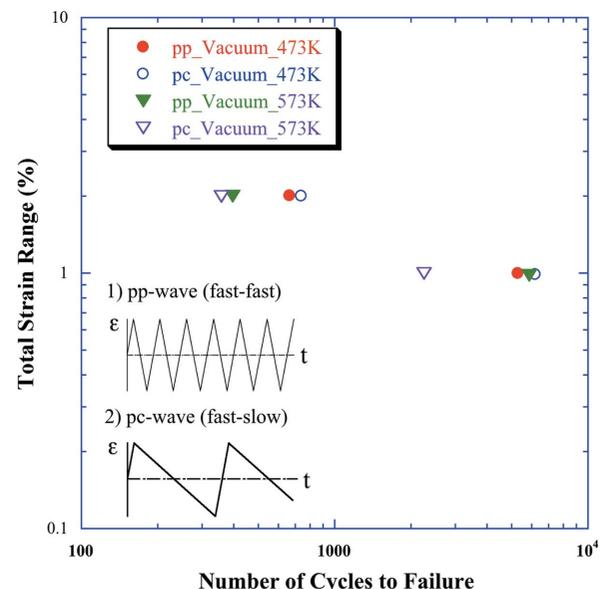
**Figure 1** Results of low-cycle-fatigue test in a vacuum. The effect of strain waveform on low-cycle-fatigue life is shown.
