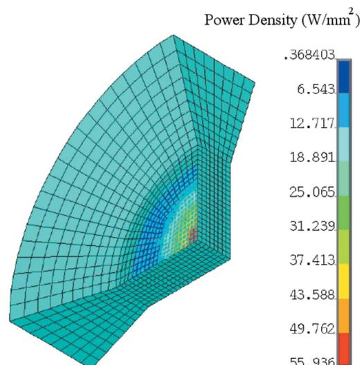
**Figure 7** Spatial distribution of the heat flux in the model. The heat flux is given as the surface load on each element.
