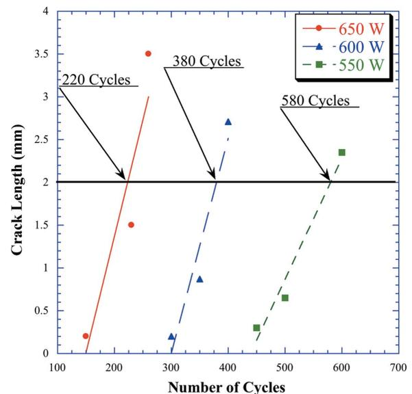
**Figure 6** Relationship between the crack length and the number of cycles for absorbed power of 550 W and 650 W.
