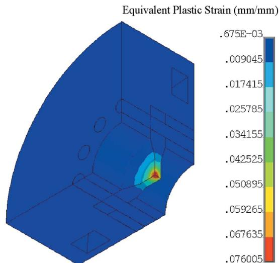
**Figure 10** Contour plot of the equivalent plastic strain just before the eighth irradiation was stopped.
