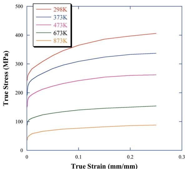
**Figure 9** Temperature-dependent stress–strain diagrams in the plastic strain region of the GlidCop body.
