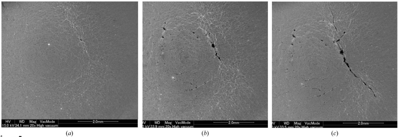
**Figure 5** Twenty magnified FE-SEM photographs of the area around the center of the test piece for an absorbed power of 650 W. (a) After 150 cycles, (b) after 230 cycles, (c) after 260 cycles.
