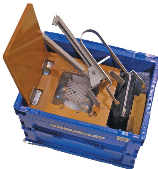
Figure 3 Overview of the compact toolkit designed for mounting crystals by hand.
