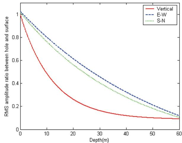
**Figure 8** Fit curves of RMS displacement ratio between the hole and surface (with truck).
