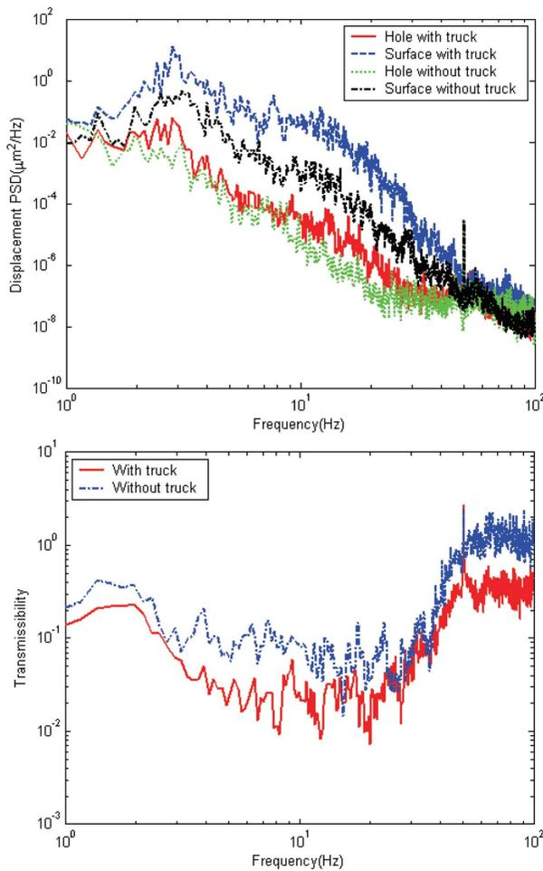
**Figure 6** Vertical vibration at a depth of 50 m: (a) displacement PSD ( $\mu\text{m}^2 \text{Hz}^{-1}$ ); (b) transmissibility from ground surface to hole.
