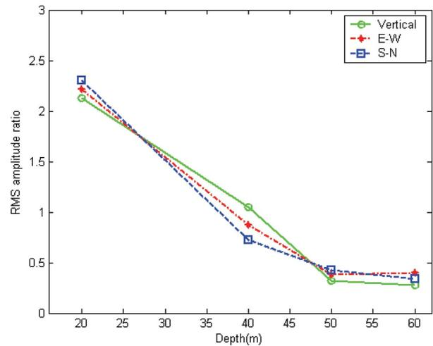
**Figure 7** RMS displacement ratio between the hole with the truck and the surface without the truck.
