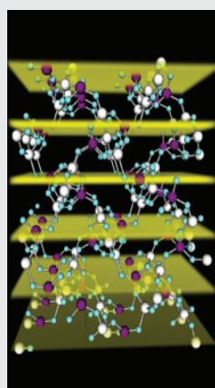
The structure of zeolite scocelite, showing the aluminium and silicon atoms as the large sphere, connected by oxygen atoms in blue. The experiment provides the distribution of aluminium and silicon within the crystal, yielding insights into the location of the active sites in a zeolite. Credits: J. Van Bokhoven.
