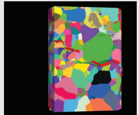
*Different visions of the cracks forming in a stainless steel wire. In the first image, the sample is visible, as well as some cracks. In the middle one, the cracks inside are coloured red, and the last picture shows the different grains that make the wire, as well as the crack, superimposed, in red, that starts to form following grain boundaries. Credits: Andrew King.*
