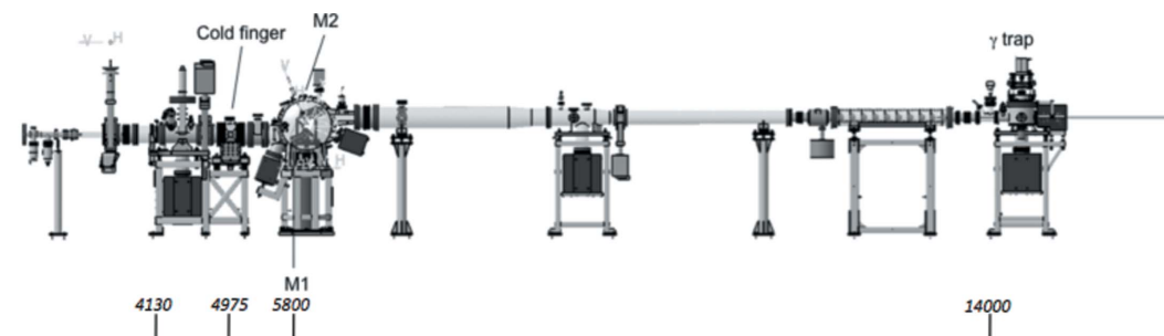
Figure 4 Layout of the DISCO beamline front-end at SOLEIL. Distances from the source point are indicated in mm for some elements.
