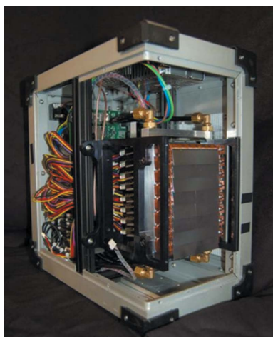
Figure 14 Silicon XPAD3S imager.
