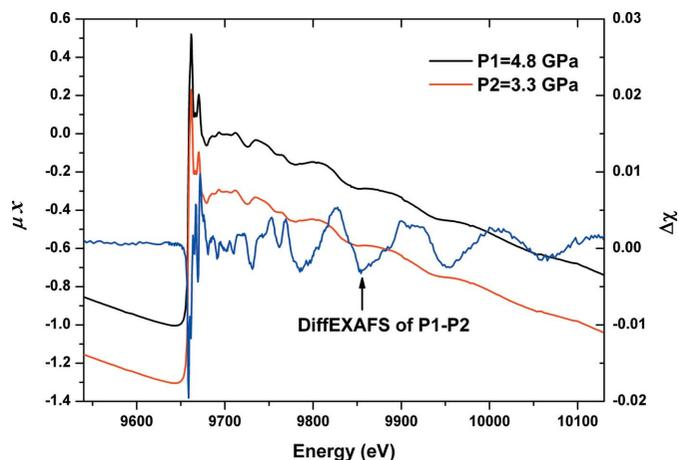
**Figure 3** Results of the measurement of Zn  $K$ -edge DiffEXAFS in ZnSe at 4.8 GPa with  $\Delta P = 1.5$  GPa.
