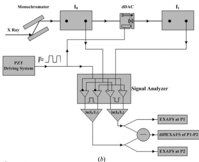
**Figure 2** (a) Modulation signal of a 1 Hz square wave. The low level corresponds to a pressure  $P_1$  on the sample and the high level to  $P_2$  ( $P_1 > P_2$ ). (b) Schematic diagram of a DiffEXAFS measurement. The square wave is divided into two parts: one part controls three PZTs, the other is a reference signal of the signal analyzer. The EXAFS spectra at  $P_1$  and  $P_2$  are obtained simultaneously, and their difference gives the DiffEXAFS spectrum.
