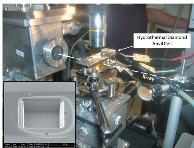
**Figure 2** The HDAC shown in the experimental set-up at beamline ID24 at ESRF, that was used to make ED-XAS measurements of Fe(II)Cl<sub>2</sub> aqueous solution samples to 773 K. The inset shows a scanning electron microscopy image of the 200 μm × 300 μm × 50 μm (depth) sample recess milled with focused ion beam into the face of a diamond anvil of the HDAC.
