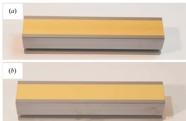
Figure 4 Photographs of M1 (a) before and (b) after atmospheric pressure UV/ozone cleaning at 363 K for 10 min. The light brown area on M1 before the cleaning was speculated to be graphite-like carbon with a flat-on configuration and a thickness of about 4 nm (see §3.1).
