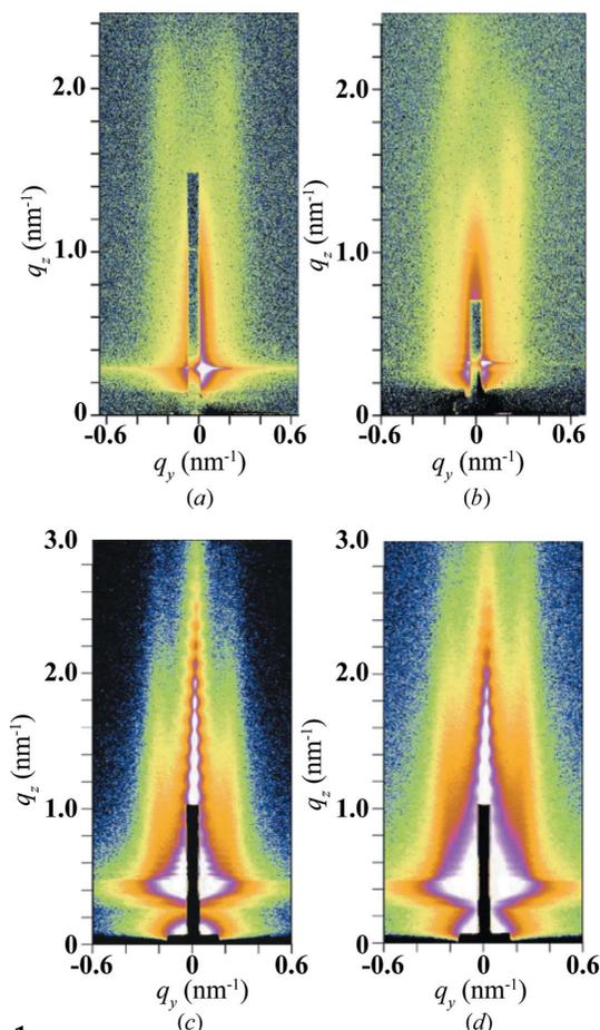
**Figure 1** GISAXS patterns of Si-capped Ge nanodots in SX and HX regions. (a)  $\varphi = 0^\circ$  for SX, (b)  $\varphi = 22.5^\circ$  for SX, (c)  $\varphi = 0^\circ$  for HX, (d)  $\varphi = 22.5^\circ$  for HX.
