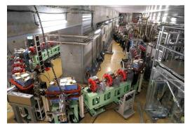
from which the electron beam is extracted. This beam is first accelerated up to 2.9 MeV by a super conducting cavity for injector, and the receives further acceleration up to approximately 20 MeV by a main cavity. We are now in the phase of improving the beam performance toward a full operation at 35 MeV and 10  $\mu$ A, through machine adjustment.
