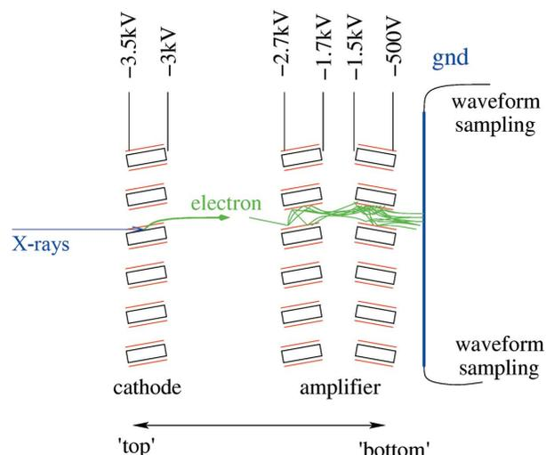
**Figure 1** Schematic cross section of the X-ray detector with one MCP optimized as an X-ray photocathode and two more to amplify the photoelectron pulses.
