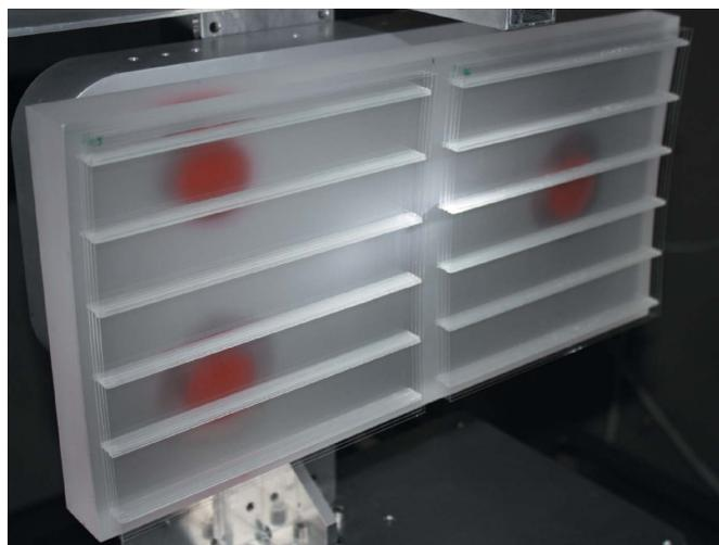
**Figure 1** An optical module, manufactured at INAF/OAB, made of four stacked pairs of slumped glasses (after Civitani *et al.*, 2013). Each pair is a grazing-incidence parabola–hyperbola system operating two reflections in sequence. Ribs are used to properly space the mirrors and to endow them with the required stiffness.
