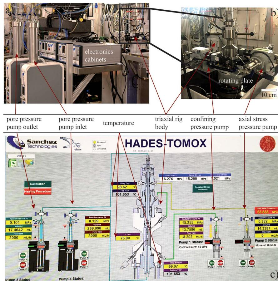
**Figure 2** HADES triaxial deformation rig installed on beamline ID19 at the ESRF. (a) View of the equipment with the rig, the electronics and the pore pressure pumps. (b) Main body of the rig shown in Fig. 1. (c) Graphical user interface for the controls. Arrows point to the various components of the equipment and their counterparts in the graphical user interface.
