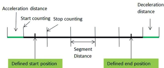
Figure 2 Synchronized continuous-scan motor position and collected data.
