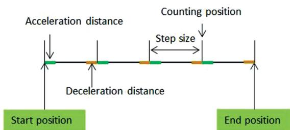
Figure 3 Step-scan motor position and data position.
