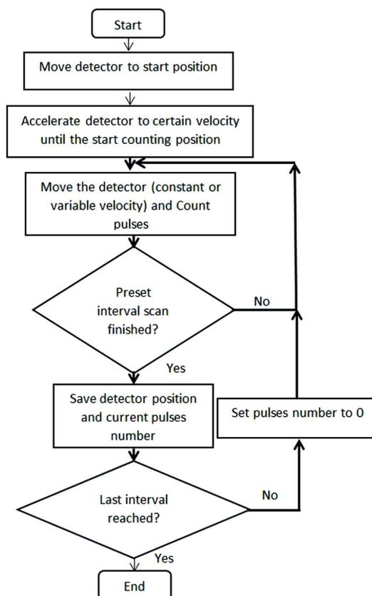
Figure 4 Flow chart for continuous scan.
