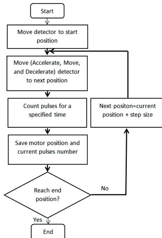
Figure 5 Flow chart for step scan.
