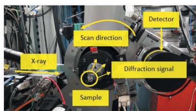
tions can decrease the signal quality by blurring the peaks. To decrease the effect of the vibrations, a settling time can be introduced, which will allow for the system to come to rest, but increases the data collection time.
