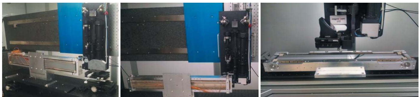
Figure 5 XDMs are inspected with our stitching Shack–Hartmann system in the NSLS-II metrology laboratory.
