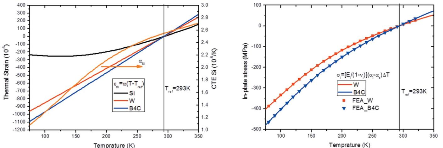
Figure 3 Non-linear CTE of Si and thermal strains of Si, W and B<sub>4</sub>C (left), and in-plane layer stresses versus temperature with T<sub>ref</sub> = 293 K (right), showing results compared between FEA and theoretical calculation.
