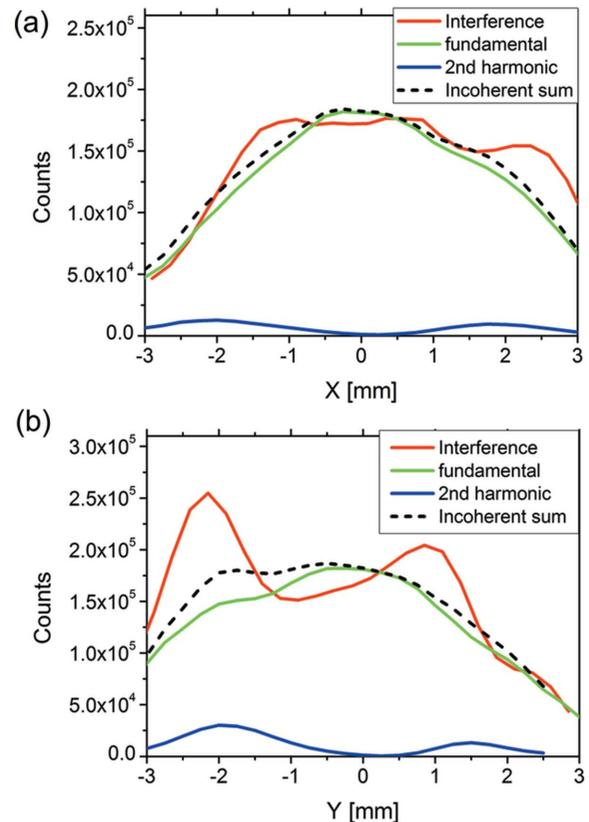
**Figure 3** Intensity profiles of photon beams at 60 nm wavelength, measured by the pinhole scan. The intensity profiles along the (a) horizontal and (b) vertical axes are derived from the two-dimensional distributions shown in Fig. 2.
