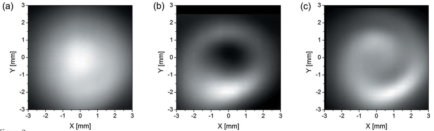
**Figure 2** Spatial intensity distributions of right circularly polarized beams at 60 nm wavelength, measured by the pinhole scan in the transverse plane. Two-dimensional profiles for (a) fundamental radiation from the upstream undulator, (b) second-harmonic radiation from the downstream undulator, and (c) interference pattern.
