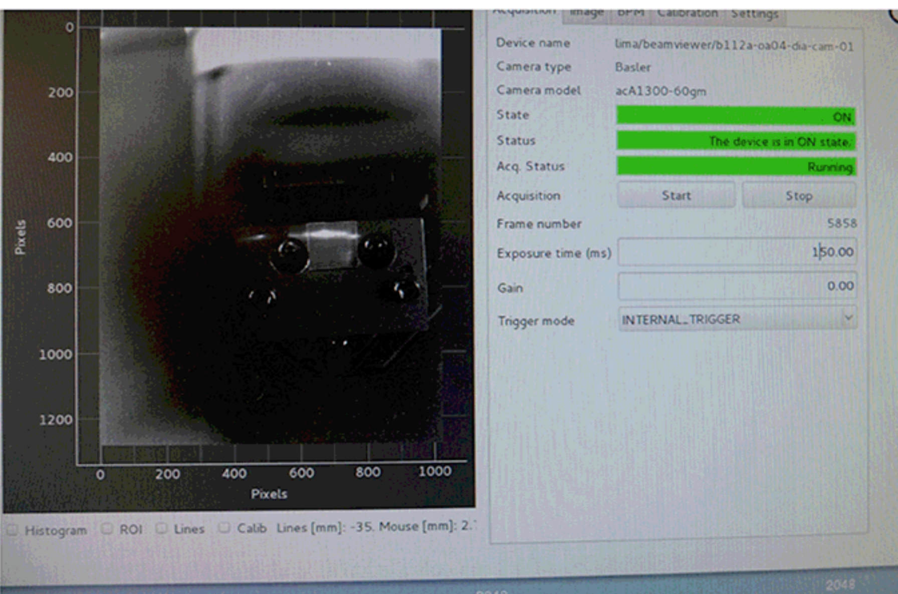
First light on exit slit of FinEstBeAMS, ring current 3.15 mA and undulator gap 75 mm.
