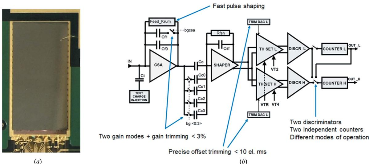
Figure 1 Picture of a single chip detector module (a) and a single pixel architecture (b).
