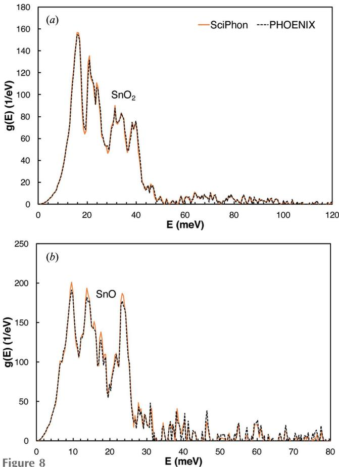
**Figure 8** Comparison between the Sn partial phonon density of states of SnO<sub>2</sub> (cassiterite; Hu *et al.*, 1999) and SnO (Giefers *et al.*, 2006) at 300 K calculated using the *PHOENIX* (dashed black curve) and *SciPhon* (solid orange curve). There is excellent agreement between the two, demonstrating that *SciPhon* can handle data reduction of Mössbauer isotopes other than iron.
