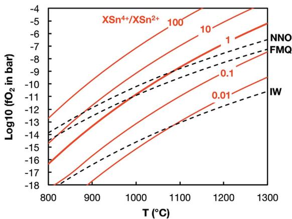
**Figure 11** Proportions of  $\text{Sn}^{4+}$  and  $\text{Sn}^{2+}$  in  $\text{Na}_2\text{O} \cdot 2\text{SiO}_2$  glass (Johnston, 1965) as a function of oxygen fugacity ( $f\text{O}_2$ ) and temperature [equation (66)]. Several oxygen buffers are shown; NNO = Ni–NiO, FMQ = fayalite–magnetite–quartz, IW = iron–wüstite. Most terrestrial igneous rocks have oxygen fugacities within  $\pm 2$  Log-units of the FMQ buffer, where  $\text{Sn}^{4+}$  and  $\text{Sn}^{2+}$  could co-exist.
