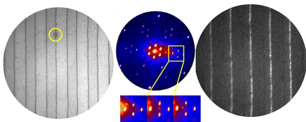
Fig.2 Bright field LEEM image ( $E=5\text{eV}$ ;  $\text{FoV}=10\text{mm}$ ), yellow circle marks the sampling area (250nm) for the micro-LEED from a single mesa wall; b) m-LEED pattern ( $E=25.5\text{eV}$ ) from a single mesa wall. Insets (bottom row) show a moving facet spot (electron energies are 25, 25.5 and 26eV, correspondingly) chosen for dark-field imaging; c) DF image ( $E=25.5\text{eV}$ ) highlighting graphene nanoribbons on every second wall of the mesa structure.
