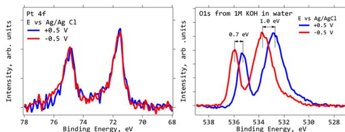
Figure 1. Pt 4f (left) and O 1s (right) XPS spectra from a 20 nm water layer on top of Pt foil. Different colors represent different applied potentials. Good overlap of Pt curves is due to grounding of the sample, whereas shift of water O1s indicates the potential is drop occurs strictly at the soli/liquid interface, thus no potential drop across the thin film.
