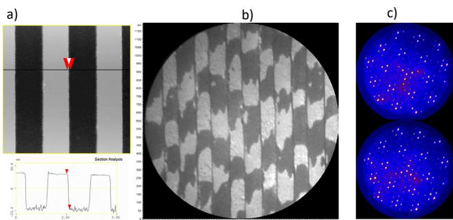
Fig.1. a) AFM image of the mesa structure after UV lithography; b) tilted bright field (TBF) ( $E=23\text{eV}$ ) LEEM image showing a nice buffer layer on the top and bottom terraces (the mesa walls are dark vertical lines) with two domains from SiC after graphene growth,  $\text{FoV}=10\text{mm}$ ; c) micro-LEED images from two domains in the TBF LEEM.
