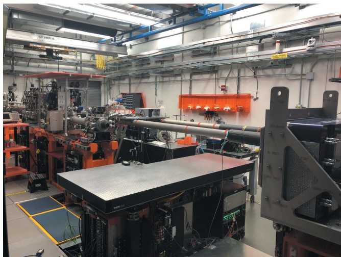
Figure 4 The MFX hutch as seen from the southeast corner. The unfocused beam enters from the left of the image, and propagates through diagnostics and slits, and continues to the transfocator and further on through more diagnostics and slits. The focused beam exits a diamond window to atmosphere towards the large breadboard of the sample table, seen here empty. To the right is the Rayonix MX340-XFEL detector on the detector mover. Above the table (not seen) is the robot arm, which can also be equipped with another smaller detector. The beam transport pipes for the MEC and CXI instruments can be seen adjacent to the MFX table.
