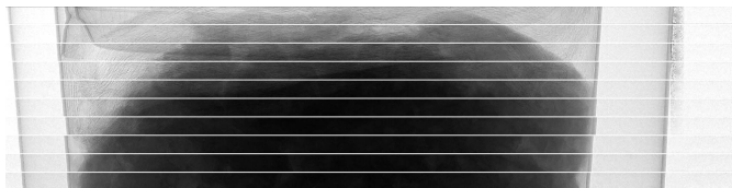
Figure 1 Collage of a sample projection for each of the ten considered vertical stages. Due to the limited vertical size of the beam, the height of each projection consists in only 51 pixels. The projections cannot be easily stitched together to compose a single projection of 510 pixels height because of the unknown angular shift and actual angular range covered induced by the continuous mode acquisition. These issues are better compensated within the reconstruction step.
