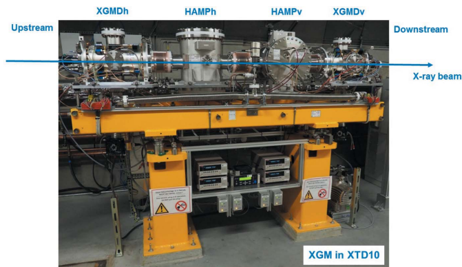
Figure 1 Photograph of the XGM in the XTD10 tunnel shown as an example. The XGM consists of four chambers: XGMDh, HAMPh, HAMPv and XGMDv. Chamber names ending with the letters h or v are dedicated for horizontal or vertical beam position monitoring, respectively.
