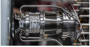
SPECIES, one of the soft X-ray beamlines in MAX IV 1.5 GeV storage ring, has added to its portfolio a new cutting-edge experimental setup. It is composed of a custom cell where the ALD process is performed and observed using APXPS. Thanks to this next-generation experimental setup, scientists can finally observe the formation of the atomic layer in real-time.
