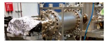
A new five-axis parallel kinematic mirror unit has been developed for MAX IV's soft X-ray beamlines. This new mirror unit was created to address the unique stability requirements of 4th-generation synchrotrons such as MAX IV. <u>Read the full story</u>
