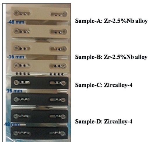
Figure 1 Photograph of samples loaded in sample containment arrangement inside the ultrahigh-vacuum chamber for TXRF measurements at the XRF beamline, Elettra Sincrotrone Trieste, Italy.
