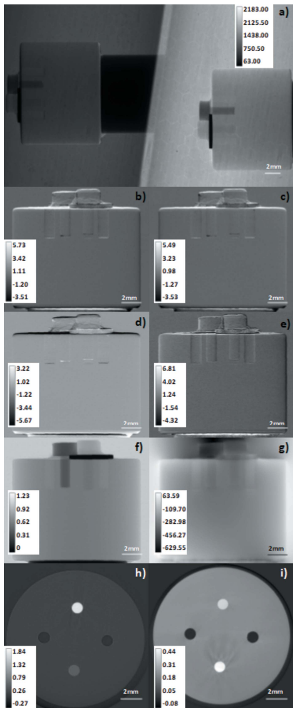
Figure 6 Maps generated throughout the experimental procedure beginning with the (a) raw tomographic data, projection number 362, showing the diffracted (left) and transmitted (right) intensities in this single projection that needs to be separated and aligned. We then perform phase retrieval to obtain maps (b) \Delta\theta' of the change of the angle of incidence upon the analyser crystal and (c) \Delta\hat{\theta}' , the 180^\circ equivalent of \Delta\theta' in microradians. From this we split \Delta\theta' and \Delta\hat{\theta}' into the (d) vertical and (e) horizontal components of the phase gradients, divided by the wavenumber, in microradians. From the transmitted projection we obtain a map of (f) intensity, while performing 2-D integration using (d) and (e) to calculate the (g) phase map in radians. We then performed tomographic reconstruction using the intensity and phase maps to calculate the (h) \beta maps ( \times 10^{-9} ), and (i) \delta maps ( \times 10^{-6} ), respectively.
