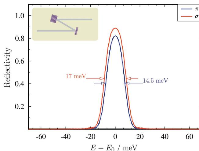
**Figure 2** Diamond crystal reflectivity for X-rays in two successive 800 Bragg reflections calculated as a function of photon energy  $E$  with a central energy,  $E_0 = 14.4125$  keV, corresponding to the nuclear resonance of <sup>57</sup>Fe. The Bragg angle is  $\theta = 74.7207^\circ$ . The photon energy dependences are calculated for two possible X-ray polarization states,  $\pi$  and  $\sigma$ .
