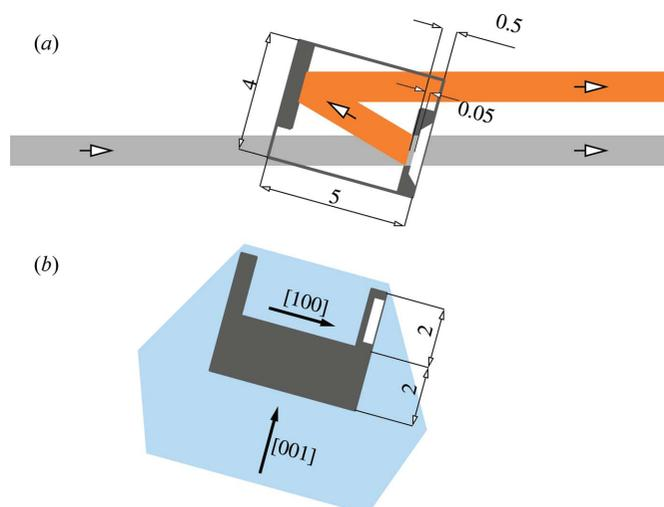
**Figure 4** Schematic diagrams of the (800) diamond channel-cut crystal monochromator for 14.4 keV X-rays (black). The channel cut is machined from an as-grown cubo-octahedral diamond crystal stone (light blue). Shown are (a) top and (b) side views with dimensions in millimetres. The propagation paths of the X-ray beams with a  $1\text{ mm}^2$  cross section are shown in panel (a).
