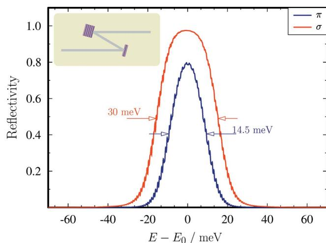
**Figure 3** Diamond crystal reflectivity for X-rays in two successive 620 Bragg reflections calculated as a function of photon energy  $E$  with a central energy,  $E_0 = 12.4$  keV, corresponding to the nuclear resonance in  $^{45}\text{Sc}$ . The Bragg angle is  $62.424^\circ$ .
