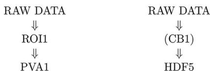
The first pipeline prepares data for broadcasting and streaming reconstruction. In case of a slow network connection or limited computing resources, one can apply binning or crop data to smaller sizes by adjusting parameters in the ROI1 plugin. The second pipeline is associated with on-demand data capturing to an HDF5 file located on the machine controlling the detector. As opposed to the first pipeline, no data binning or cropping is applied in this case.
