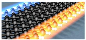
An international research group found epitaxial zigzag graphene nanoribbons grown on mesa-structured silicon carbide form protected spin-polarized transport channels, without the application of an electromagnetic field. Their results hold potential for the advancement of spintronics. <u>Read the full story</u>
