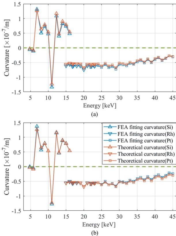
**Figure 5** Comparison between theoretical curvatures and FEA fitting curvatures. The green dashed line shows where the curvature equals zero. (a) FEA fitting curvatures without calculating  $c_0$  and (b) taking  $c_0$  into account.
