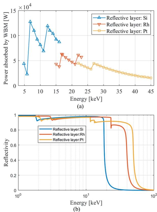
**Figure 2** (a) Power absorbed by the WBM at different photon energies. The range of the fundamental harmonic is from 4.8 keV to 6.8 keV, the range of the third harmonic is from 6.8 keV to 11 keV, the range of the fifth harmonic is from 12.3 keV to 26 keV, and the range of the seventh harmonic is from 27 keV to 45 keV. (b) Reflectivity curve of the Si, Rh and Pt layers.
