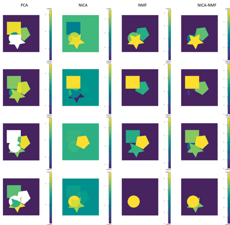
Figure 7 Example of blind source separation. Each column corresponds to a BSS method: PCA, NICA, NMF, NICA–NMF. The found components are shown for each method.
